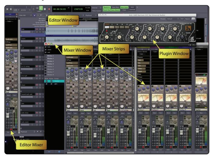
A Mixer Strip is a vertically-aligned group of controls which affect a single track or bus.
